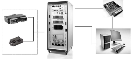
Osswald et al. (2013). Hardware-in-the-Loop-Based Evaluation Platform for Automotive Instrument Cluster Development (EPIC).
